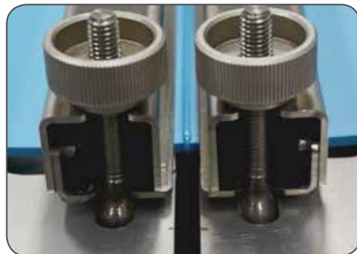
Welded splice prior to skiving bead
