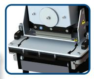
Belt Clamps on edge of support table **SECURE VARIOUS PROFILED BELT** in place.
