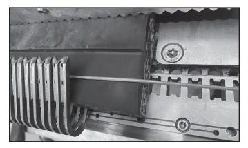
Load the XP<sup>™</sup> Staple Fasteners in the bed, centre the belt between the fasteners, and tighten the clamp bar. Insert the end plate in one of the H-holes on the left-hand side of the bed and thread the XP-LOK<sup>™</sup> Belt Wire through. Tension the wire by using the thumb screw. Only tension the wire until finger tight.
