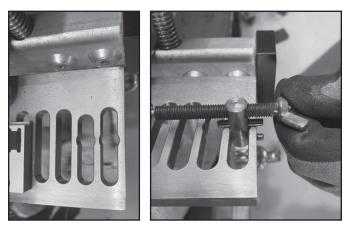
3. The XP-LOK<sup>™</sup> wire should be tensioned to the centre of the fasteners and belt. Install the fasteners. Monitor the tension and position throughout the entire installation, make adjustments as necessary. Use wire cutters to cut any excess wire if necessary. Loosen the thumb screw, remove the end block and screw tensioning rod, and release the belt from the clamp bar.
