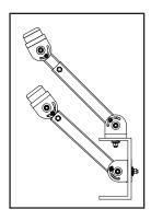
2. Using the mounting base as a template, mark and proceed to burn/drill mounting holes. Mounting holes may already be present on the conveyor structure. Install mounting base and tighten hardware.
