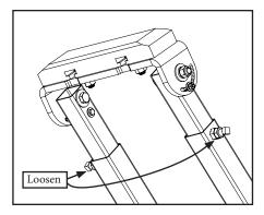
3. Loosen bolts and remove the worn UHMW bar.
