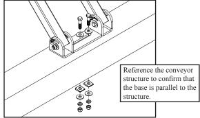
**NOTE:** Unit may be disassembled at the telescoping tubes for additional ease of installation, but is not necessary. If disassembled, reassemble prior to next step. Do not tighten hardware.
