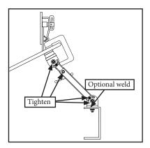
5. Remove c-clamp or quick clamp and check all hardware for tightness. Repeat on oppsite side of conveyor.
