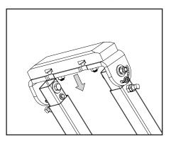
4. Replace the UHMW bar and retighten the bolts.
