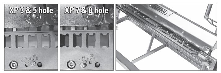
1. Insert belt end into frame centered on the bed and until it rests against all belt stops. Tighten clamp bar.
