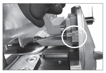
**3.** Adjust blade holder to desired cutting depth. Ensure blade adjustment handle is in the up position prior to skiving.
