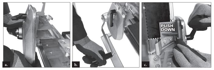
**2. a.** Attach the skiver to the bed by sliding the mounting bracket onto the left side of bed rail. **b.** Turn Drive Handle clockwise to engage the skiver with the bed. Raise Upper Pressure Plate. Move skiver over belt until Upper Pressure Plate is positioned about 50 mm (2") over the belt. **Ensure blade is not touching the belt. c.** Push Upper Pressure Plate firmly down against belt surface and tighten Adjustment Lever to lock in position.
