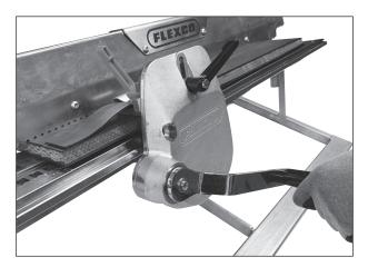
**4.** Turn Drive Handle clockwise to begin skiving. Make sure scrap cut does not get jammed in skiver. Spraying silicone on belt will reduce required effort. **If effort is high, stop, reverse and inspect for loose or damaged parts.**
