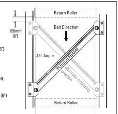
Physically lock out and tag the conveyor at the power source before you begin plough installation.
