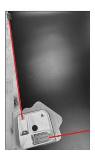
5. Align the laser that is directed down the length of the belt with the belt edge. Maintain contact with one of the 2 pins on the template with the LBS as well as maintain contact between the bottom side template pin and the edge of the belt.
