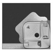
2. Locate the pin on the underside of the bias template. Position the bias template so this pin makes contact with the edge of the belt.
