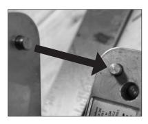
1. Align the largest pin on the Bias Template Tool with the pin on the LBS and press them together. The LBS should sit on top of the Bias Template Tool. Do this so that the tool can swivel and contact each of the smaller pins.
