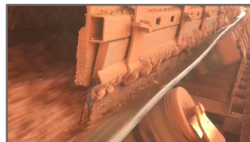
Flex-Lok™ sealing system with Polyurethane skirting.
