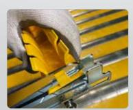
**Transfer Plate Cutter** to cut transfer plate to length
