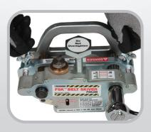
Easily adjust fence for the appropriate fastener size.
