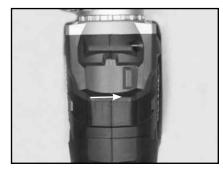
3. Cutting Speed Adjustment; adjust Electric Drill to low speed by moving switch to low speed. For best results, always operate skiver in low speed.
