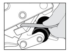
2. Using flat side of sharpening stone, sharpen bevel on the top-side of the blade.
