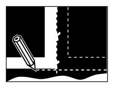
1. Cut belt using centerline method. NOTE: For easier skiving, clean belt and use only sharp, undamaged blades.
