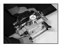
8. Advance skiver in a controlled manner across width of belt. Ensure belt is against Fence. Advance skiver completely off belt to complete cut. Remove scrap cut. Repeat steps 1-8 on other belt end.
