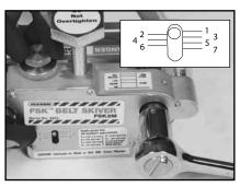
2. For new tool, carefully remove the protective coating on the blade. Turn Blade Adjusting Screw to select desired cutting depth. Tighten Jam Nut.
