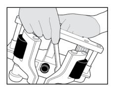
Changing the Blade: Turn blade adjusting screw to raise blade and turn clamp adjusting screw to lower grip rollers. Using a  $\frac{7}{16}$  box type wrench, remove the  $\frac{1}{4}$ -20 bolt from the blade holder.
