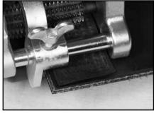
7. When skiving, scrap cut should remain in contact with belt. Scrap cut and Belt should feed under Rear Drive Rollers.
