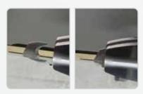
*Cutter Storage Position: Cutter must be in storage position for splicing function to operate.*
