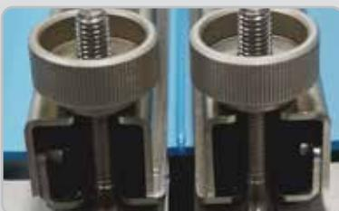
**Cool Zone:** Heater stows and cools inside unit as belt ends are butt-welded together.
