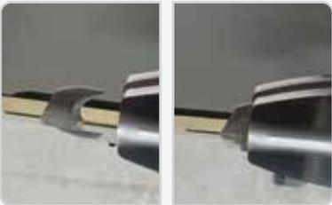
**Cutter Storage Position:** Cutter must be in storage position for splicing function to operate.
