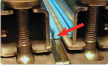
**Integrated Cutter:** Operator is protected from blade during single pass cutting operation.
