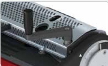
**Shielded Heat Zone:** Guard must be closed for heat emitter to function. Operator is protected from heat source during splicing.
