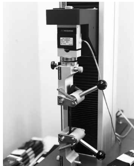
Quality Engineer conducting test ASTM-D429 at Flexco Australia's Internal Cold Bond Testing Facility.
