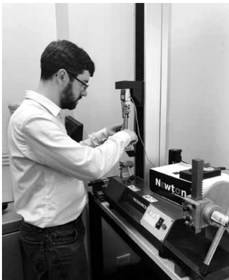
Quality Engineer conducting test ASTM-D429 at Flexco Australia's Internal Cold Bond Testing Facility.
