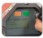
Utilizes **BLUETOOTH® TECHNOLOGY** to access and evaluate splice data and manage updates to firmware for ongoing press enhancements.
