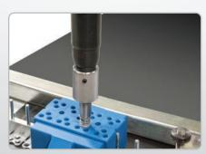
Air Powered Rivet Driver Installation
