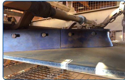
Freshly installed blades on existing V-plough frame
