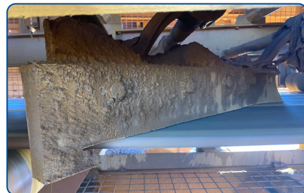
Blades after 12 months, displaying only 40% wear
