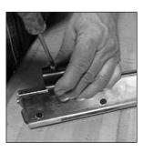
**6.** Finish tightening the screws until the bottom of the head just touches the top of the springs.
