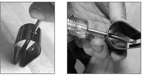
**2.** Insert a small straight edge screwdriver and rotate to open spring as shown.
