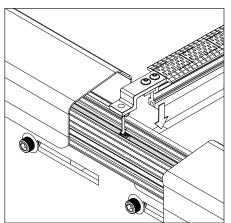
5. Position the Narrow Gap STP as normal using the carboard shims. Reference Narrow Gap Segmented Transfer Plate IOM (X4657) for full installation details. Note: Do not let the Narrow Gap STP or bracket rub against the drive belt.
