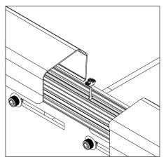
4. Place the Hammer Nut in the channel and attach the bracket to the hammer nut using the button head screw.
