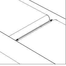
2. Measure the width of the conveyor structure and cut the Narrow Gap STP aluminum bar 1/8" less than the width.
