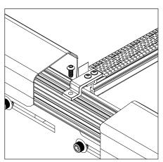
6. Once the Narrow Gap STP is in its final position, tighten all fasteners. Verify proper clearances between the segments and incoming belt, and the Narrow Gap STP and drive belt.
