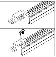
3. Assemble the bracket and nut plate, into the Narrow Gap STP aluminum bar.
