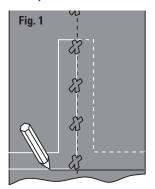
1. Square belt using centerline method and mark a perpendicular line across the belt. OR if installing on a pre-cut belt, ensure both ends are square.
