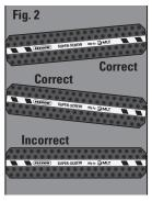
2. Lay the splice face up on the belt to visualize the bias. This will help determine where to draw the bias and cut the belt. The face of the splice has circular indents in the rubber where the screws will be installed. Super-Screw Primary splices can be installed with the bias in either direction.
