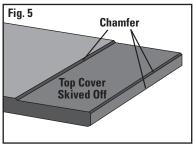
5. Chamfer the top cover on the trailing side of the belt. Then chamfer or bevel the top and bottom edges of both ends of the belt.
