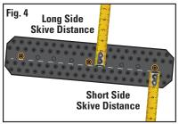
4. Using Table A on the back, or measuring from the spacers perpendicular to the edge of the strip, determine the distance to skive on each end of the belt. **Note:** The measurement will be different on each end of the belt. Skive off as much top cover rubber as possible without cutting into the plies of the belt. It is recommended to skive the bottom cover if it is greater than one eighth (1/8") of an inch.
