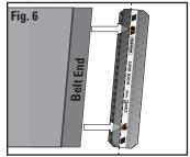
6. Centering the splice on the belt, slide the strip onto the end of the belt with the shorter skive reachback. Ensure belt is firm against all of the pre-inserted spacers.
