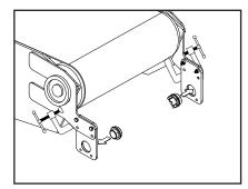
**2.** Trim brackets as necessary, then temporarily clamp brackets to conveyor structure. This will allow for future adjustments.
