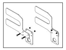
**1.** Bolt or clamp Y brackets to the mounting plates included with the cleaner assembly. A minimum of two bolts is required if bolting. Position Y bracket on conveyor structure so that the shaft hole of the mounting plates meets the X, Y, and C dimensions, per the cleaner IOM.
