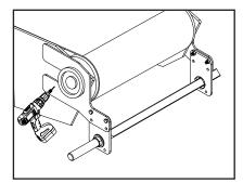
**4.** If the pole is in the correct position, bolt or weld Y brackets to each side of the conveyor.
