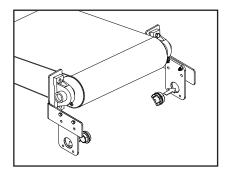
**2.** Trim brackets as necessary, then temporarily clamp or tack weld brackets to conveyor structure. This will allow for future adjustments.
