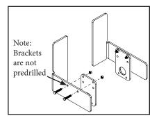
1. Clamp the 90-degree brackets to the mounting plates included with the cleaner assembly. Position 90-degree bracket on conveyor structure so that the shaft hole of the mounting plates meets the X, Y, and C dimensions, per the cleaner IOM.
