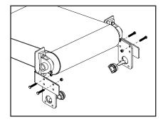
**5.** Bolt mounting plate to bracket on each side of conveyor if not done in step 1. A minimum of two bolts is required
