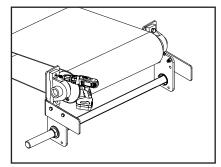
**4.** If the pole is in the correct position, bolt or weld brackets to each side of the conveyor.
