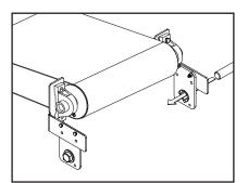
**3.** Test fit cleaner without blade. Pole should be parallel to the pulley.
