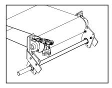
**4.** If the pole is in the correct position, bolt or weld brackets to each side of the conveyor.
