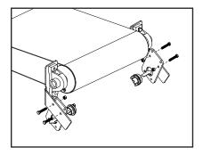
**5.** Bolt mounting plate to bracket on each side of conveyor if not done in step 1. A minimum of two bolts is required
