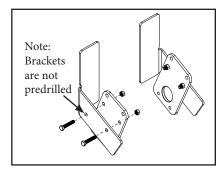
1. Clamp the sloped brackets to the mounting plates included with the cleaner assembly. Position sloped bracket on conveyor structure so that the shaft hole of the mounting plates meets the X, Y, and C dimensions, per the cleaner IOM. Drill holes on the sloped brackets and secure the mounting plates to the brackets with hardware.
