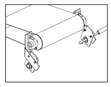
**3.** Test fit cleaner without blade. Pole should be parallel to the pulley. Reference IOM X5013 for mounting.
