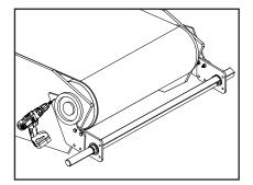
**4.** If the pole is in the correct position, bolt or weld V brackets to each side of the conveyor. **NOTE:** When bolting, at least two bolts must be used per side.
