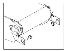
**2.** Position V bracket on conveyor structure so that the shaft hole of the mounting plates meets the X, Y, and C dimensions, per the cleaner IOM. Trim brackets as necessary, then temporarily clamp brackets to conveyor structure. This will allow for future adjustments.
