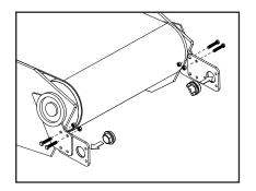
**5.** Bolt mounting plate to bracket on each side of conveyor if not done in step 1.
