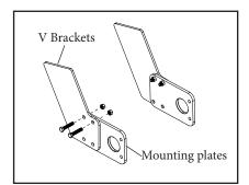
**1.** Bolt or clamp wide V brackets to the mounting plates included with the cleaner assembly.
