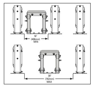
**NOTE:** The Belt Support Bar may be installed on a horizontal or vertical surface on the conveyor structure.
