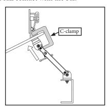
**4. Tighten the telescoping tube hardware while the unit is positioned.** Proceed to tighten the hardware on the bar base and mounting base to lock in all rotational and extension adjustment.
