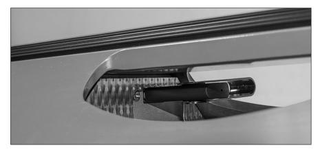
1. Follow instructions on powering up the press, then insert USB flash drive into the USB port in the top of the press.
