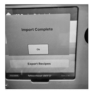
3. Once complete, the display reads "Import complete." Select "Ok," which will bring you back to "USB Device Detected." Select the back arrow to return to the home screen. At the end of updating recipes, the USB flash drive may be removed.
