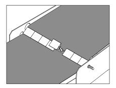
**2.** Install the segments onto the bar across the width of the conveyor. Reference installation manual X3627 for full installation details.
