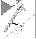
**4.** Position rotational bracket into desired installation position and clamp to the conveyor structure. Repeat for each side of the conveyor.
