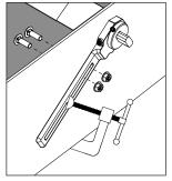
**9.** Fasten the bracket to the conveyor structure using the included bolts and washers, transfering drilling as required prior to removing the clamps.
