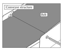
1. Use HG segments to estimate the bar location. Drill or cut a 1.5" (38mm) diameter hole through each conveyor wall, aligning the holes perpendicular to the conveyor belt. Slide the HG mount bar through each hole.
