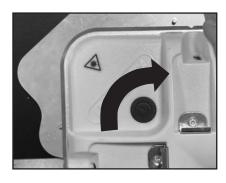
**6.** Once laser is aligned rotate the LBS without moving the template until it is in contact with the opposite pin.
