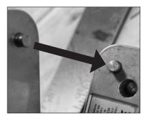
1. Depress spring loaded pin found on the bottom of Laser Belt Square (LBS) and engage with the larger of the 3 pins on the bias template. Do this so that the tool can swivel and contact each of the smaller pins.
