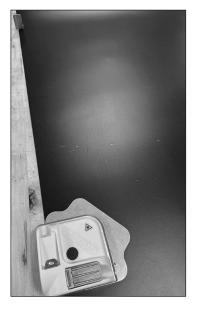
**3.** Direct the laser so that one laser spans the width of the belt and the other is directed down the intended useable belt.
