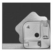
2. Place the tool and template on the belt and position it such that the pin protruding from the under side of the template is in contact with the edge of the belt.
