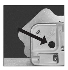
**4.** Turn the LBS on by depressing the black power switch (Caution is to be taken when directing the laser beams).
