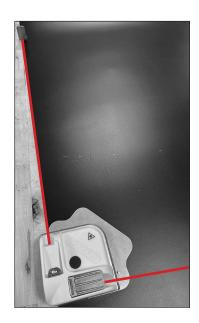
5. Align one of the lasers with the edge of the belt. Maintain contact with one of the 2 pins on the template with the LBS and maintain contact between the bottom side template pin and the edge of the belt.
