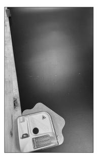
**3.** Rotate the LBS on the template so that one of the lasers is roughly directed down the length of the belt.
