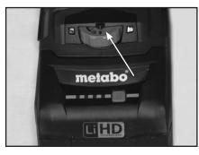
2. Operate in Maximum Torque Mode only; turn the dial to indicate drill mode.
