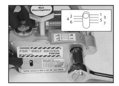
2. For new tool, carefully remove the protective coating on the blade. Turn Blade Adjusting Screw to select desired cutting depth. Tighten Jam Nut.
