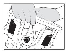
Changing the Blade: Turn blade adjusting screw to raise blade and turn clamp adjusting screw to lower grip rollers. Using a <sup>7</sup>/<sub>16</sub> box type wrench, remove the <sup>1</sup>/<sub>4</sub>-20 bolt from the blade holder. WARNING: Use caution when handling blade. Take the old blade out and replace with a new blade. Retighten bolt.
