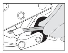
1. Using rounded side of sharpening stone, sharpen bevel on the curved portion of the blade.
