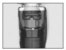
3. Cutting Speed Adjustment; adjust Electric Drill to low speed by moving switch to low speed. For best results, always operate skiver in low speed.
