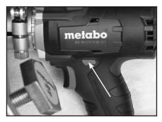
1. For normal use, operate in Reverse Direction; press drilling direction button for reverse direction operation.
