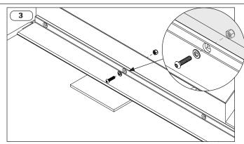
Apply fasten the Belt Edge Protector using the 1/4"-20 bolt, washer, and Nylock nuts provided, following the manufacturer's instructions. Based on the manufacturer's information, a minimum torque of 22 in-lbs is recommended. For best results, tighten each nut to contact with the structure plus one full turn.
