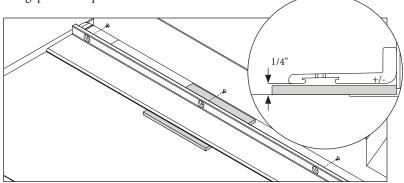
**NOTICE:** For best results, place the first Belt Edge Protector at the start of the conveyor belt and add segments until there are Belt Edge Protector segments installed along both sides of the entire length of the conveyor. Chute lip must maintain 2" height for BEP to work correctly. This product should not be installed if there is less than 2".
