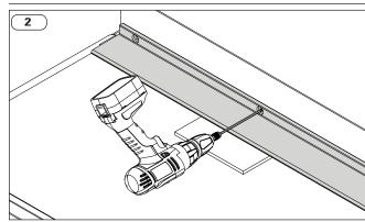
While holding the Edge Protector firmly against the sidewall, use the pre-drilled holes as a template to drill through the wall. Use both the extension bit holder and 1/4" bit while drilling.
