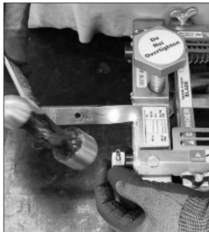
8. Insert the new spring pin.
