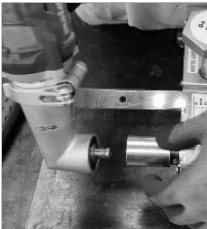
10. Remove the old drill adapter and attach the drill to the new adapter.
