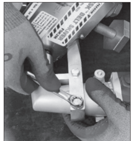
12. HAND tighten the hex bolts securely with the 7/16 wrench.
