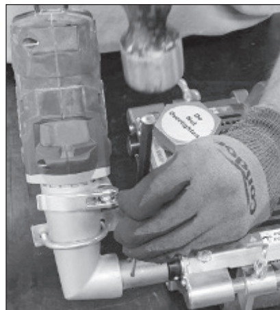
2. Drive the two small spring pins out with punch or rivet.
