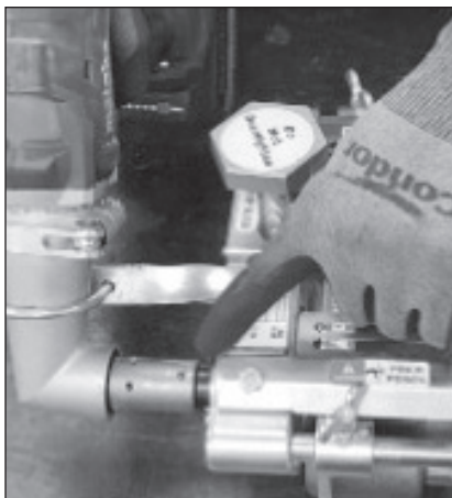
1. Position spring pins upright, then remove the battery.
