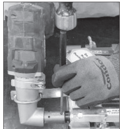
3. Drive the large spring pin out with punch or duplex nail.
