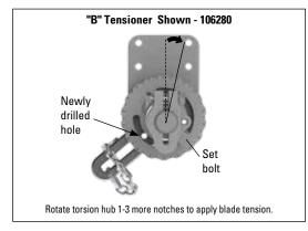
3. Set the torsion in the tensioner per the cleaner IOM, X6056 for FGS or 103689 for FGP-ES. After setting the pre-tension but before tightening the Lever clamp bolt, determine the Lever position when the blade is held away from the belt. Drill out one of the M8 threaded holes using a 5/16" (8mm) diameter drill in the Side Plate aligned with the slot of the Locking Lever.
