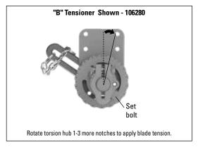
4. Position lever in accessible position roughly 30° from the new hole in the direction of the pre-tension and tighten Locking Lever clamp bolt. Ensure Locking Lever is tight on the cleaner shaft. Operate Lever to move blade away from belt and lock in place by setting the provided pin through the Lever slot and 5/16" (8mm) hole. Test run the conveyor per the cleaner IOM.
