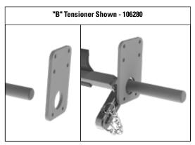
Slide the cleaner pole until the round end is inside the side plate, slide the Locking Lever onto the pole, then re-insert the pole through the side plate. Do not tighten the Lever clamp bolt.
