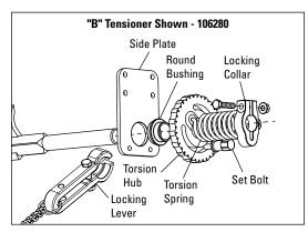
Carefully loosen and remove the tensioner set bolt, then loosen the locking collar and remove the tensioner unit from the cleaner.
