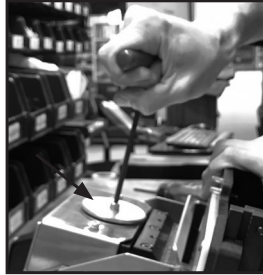
Step 2a. Remove cam guard cover.
