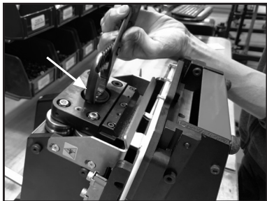
Step 4. Remove bearing (pliers may be required).
