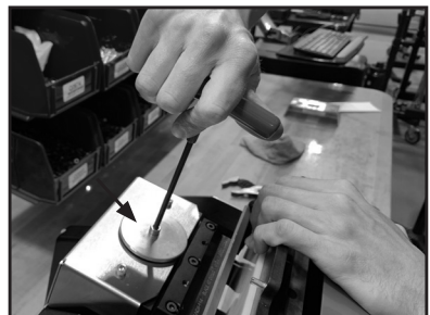
Step 8. Install new bearing spacer. Install cam guard cover over bearing spacer, securing with one fastener. Return Pun M NDX to upright position.
