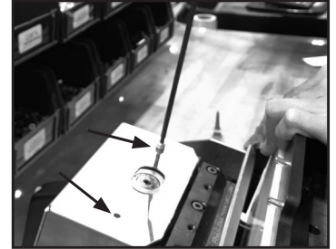
Step 3. Remove the two fasteners on the cover plate. Save for reuse. Remove cover plate.
