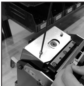
Step 7. Install new cover plate. Secure with the two fasteners removed in Step 3.
