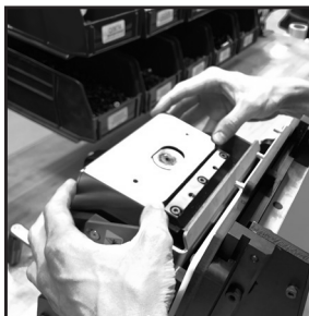
Step 7. Install new cover plate. Secure with the two fasteners removed in Step 3.
