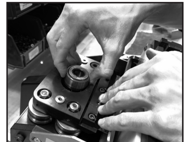
Step 6. Install new bearing (rubber mallet may be required).
