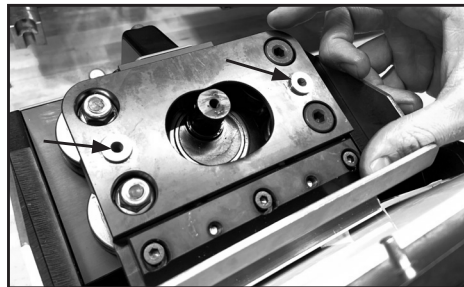
Step 5. If necessary, replace cover plate spacers on either side of blade holder assembly.
