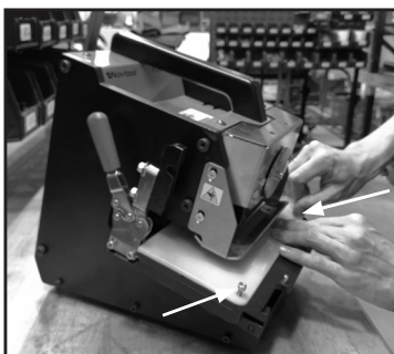
Step 16. Reinstall punch pad by securing two fasteners at front corners of pad.
