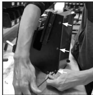
Step 13. Secure the bottom plate by screwing in the three fasteners on each side of punch.
