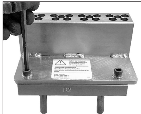
4. Reattach locator block using original socket head cap screws.
