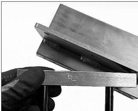
3. Flip locator block 180° so R2 is visible.
