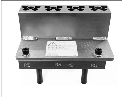
1. Original R5, R5-1/2, R6 locator block position.
