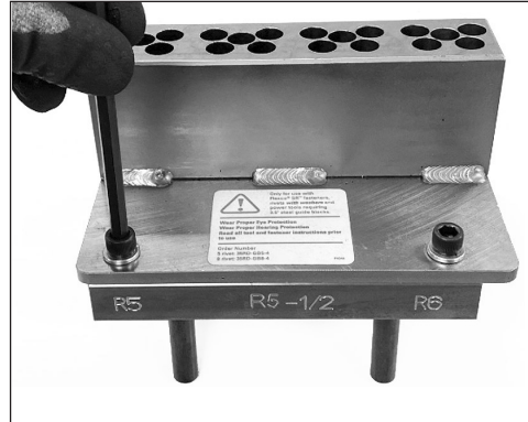
2. Remove two socket head cap screws using 1/4" Allen wrench.
