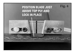
5. Carefully adjust the blade depth by sliding it in or out of the clamps. It is recommended to skive off as much of the belt's top cover as possible, while making sure to avoid cutting into the plies of the belt. Hold the handle with the brass head on the edge of the belt and set the blade to just above the top ply (Fig. 4). Use the Allen wrench to lock the set screws to the desired depth.
