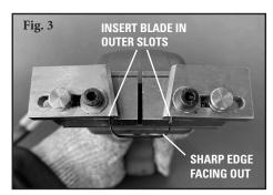
**4.** Insert a blade (sharp side facing away from the handle) into the outer slots in the spring-loaded clamps (Fig. 3). The sharp side faces forward as you push the handle away from you.
