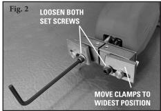
3. Using the 4 mm Allen wrench, loosen the two set screws in the brass head and move the spring-loaded clamps all the way to the widest position (Fig. 2). It is recommended to store the Allen wrench in the black rubber band wrapped around the yellow cords to avoid losing it.
