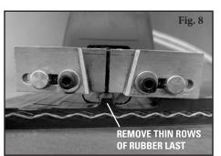
9. Lower heat setting to 1 and go back and remove the small rows of rubber left between passes (Fig. 8 and 9).
