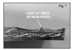
8. Continue skiving the belt, leaving 1/8" of space between passes (Fig. 7). This helps prevent the blade from overheating (turning red, warping, and breaking).
