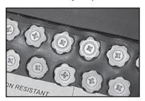
How tight do I set the screws? Tight enough so that there is a small belt pucker around the washer.
