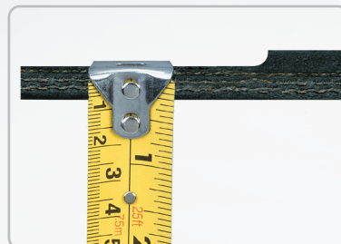
Measure belt thickness after skiving
