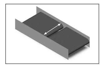
2. Measure the inside structure width to determine the placement of the bracket.
