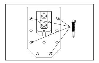
4. Secure the bracket with at least four fasteners.
