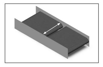
2. Measure the inside structure width to determine the placement of the bracket.
