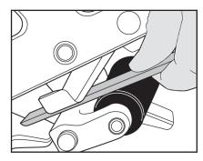
3. Using flat side of sharpening stone, sharpen bottom edge of blade flat.
