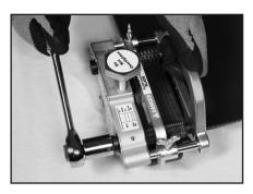
6. Note skive direction and set tool to reverse. Once belt reaches Rear Drive Rollers, turn Clamp Adjusting Screw counter-clockwise 1/4 rotation.
