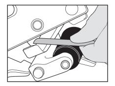
2. Using flat side of sharpening stone, sharpen bevel on the top-side of the blade.
