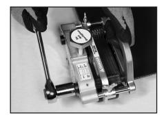
6. Note skive direction and set tool to reverse. Once belt reaches Rear Drive Rollers, turn Clamp Adjusting Screw counter-clockwise 1/4 rotation.
