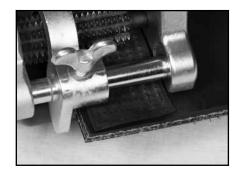
7. When skiving, scrap cut should remain in contact with belt. Scrap cut and Belt should feed under Rear Drive Rollers.
