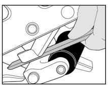
3. Using flat side of sharpening stone, sharpen bottom edge of blade flat.
