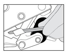
1. Using rounded side of sharpening stone, sharpen bevel on the curved portion of the blade.
