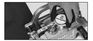
4. Turn Clamp Adjusting Screw counter-clockwise to loosen grip rollers. Position edge of belt against Fence – belt should just touch blade edge.
