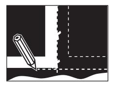
1. Cut belt using centerline method. NOTE: For easier skiving, clean belt and use only sharp, undamaged blades.
