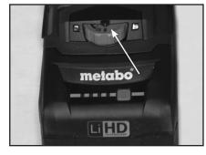
2. Operate in Maximum Torque Mode only; turn the dial to indicate drill mode.
