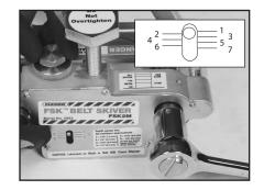
2. For new tool, carefully remove the protective coating on the blade. Turn Blade Adjusting Screw to select desired cutting depth. Tighten Jam Nut.
