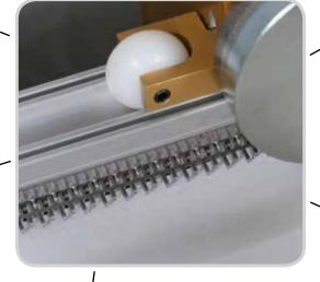
**Flat, Low-Profile Splice** is ideal for applications with slider beds
