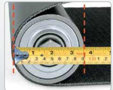
Measure smallest pulley diameter.
