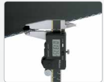
Measure belt thickness.
