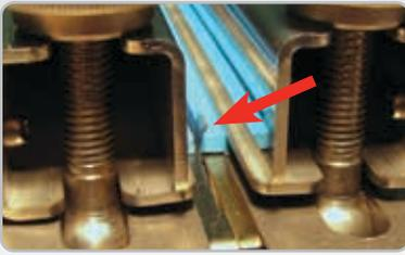
**Integrated Cutter:** Operator is protected from blade during single pass cutting operation.
