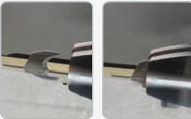
**Cutter Storage Position:** Cutter must be in storage position for splicing function to operate.
